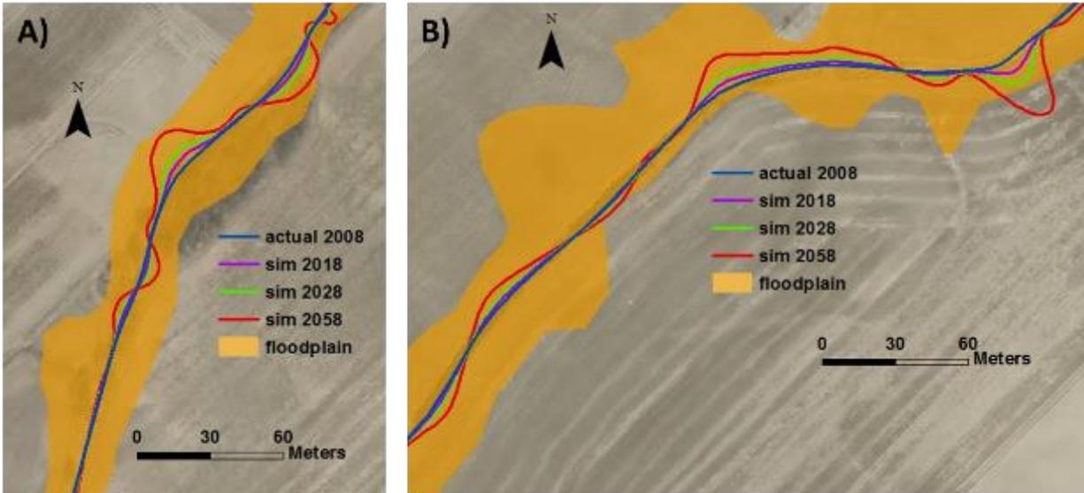
Figure 68: RVR Meander simulation results for DF using the actual input parameters for A) upstream section, B) downstream section
