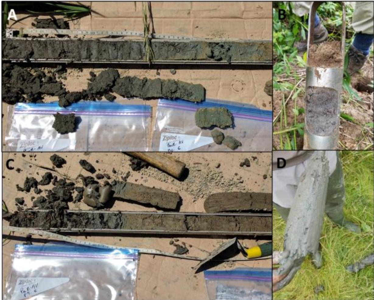
**Figure 20: A) example of a transition area between stratigraphic units from a sample extracted at PPauB; clear contact depth between units for a sample extracted at RM B) and PPauB C); D) basal unit of marine clay at DF.**
