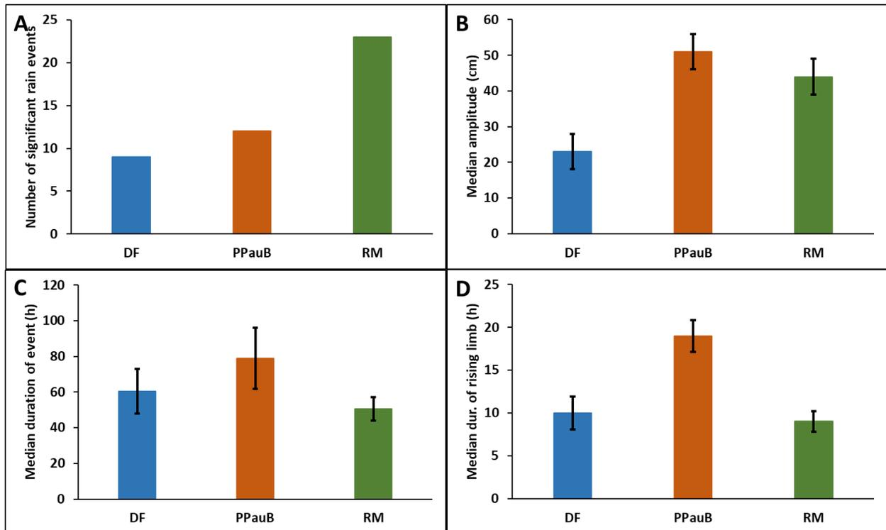
**Figure 33: Comparison of channel response to significant rain events between the three sites. A) total number of events from October 2017 to November 2018; B) Median amplitude (initial stage to peak); C) Median duration of event (time to return to baseflow conditions or another event started); D) Median duration of the rising limb (time to peak water level in channel).**
