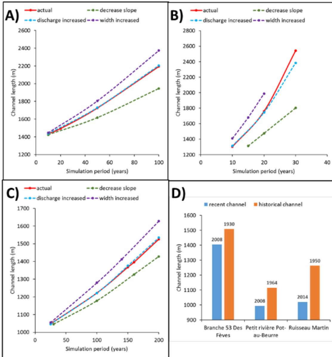
Figure 74: Comparison of channel lengths across different time periods and scenarios simulated in RVR meander for A) DF, B) PPauB, C) RM; as well as D) comparison of channel length between pre- and post-channel straightening intervention.
