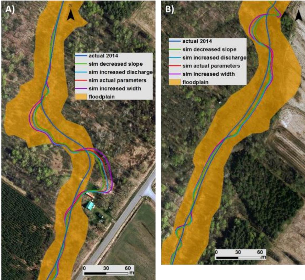
Figure 73: RVR Meander results for RM simulating actual and adjusted parameters over 100 years (2114) for A) upstream section, B) downstream section.
