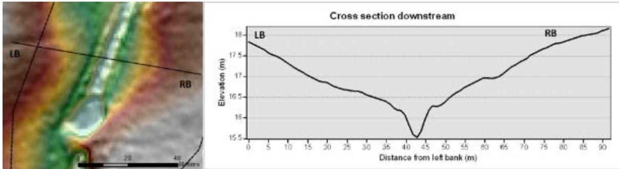
**Figure 10 : Cross-section extracted from the LiDAR highlighting disconnection from the ancient meander in the downstream reach of PPauB.**
