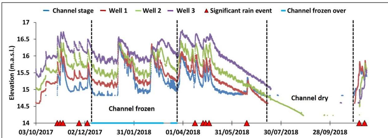
Figure 35: Channel, groundwater levels and significant rain events as a time series over the study period taken at the downstream gauging station at PPauB.
