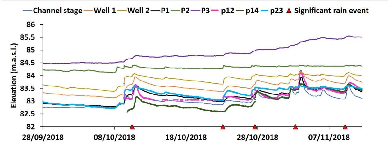
Figure 40: Channel, groundwater levels and significant rain events as a time series for the fall period (including piezometers added) taken at the upstream gauging station at RM left bank.
