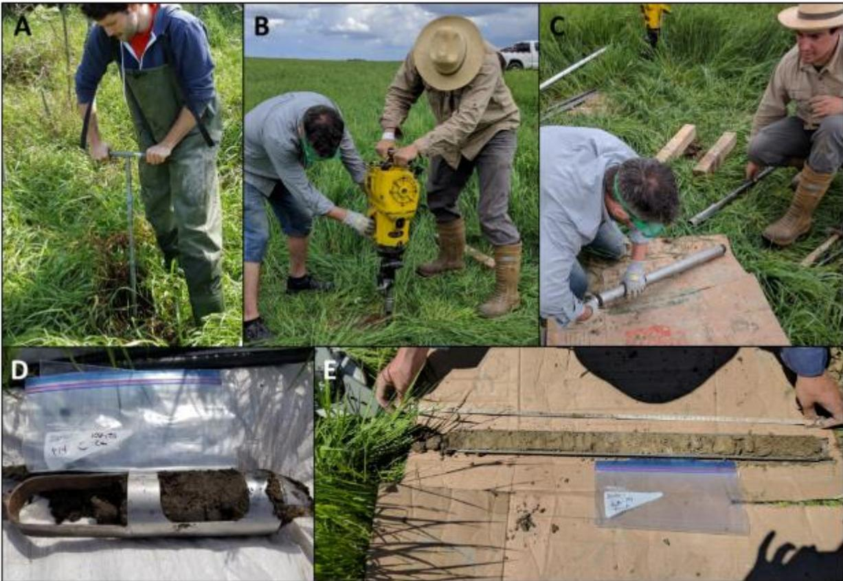
**Figure 19: A) Borehole dug at DF using auger; B) borehole dug at PPauB using Pionjar; C) 1m core sample extracted by the Pionjar; D) soil sample extracted with the auger; E) soil sample obtained from Pionjar.**
