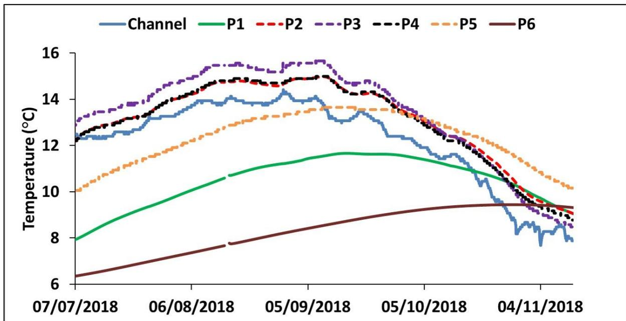
**Figure 51: Temperature data of channel and groundwater collected at RM mid for the summer/fall period of 2018. Dashed lines indicate piezometers installed in the topographic depression associated with the ancient meander.**
