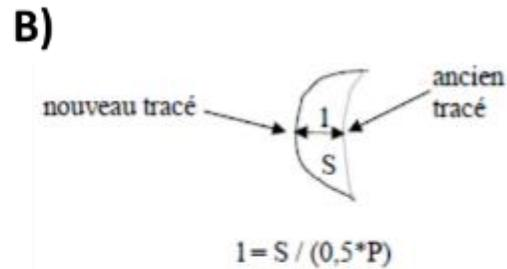
Figure 65: A) Example of determination of channel migration from historical channel position in 1960 to 2014 for Ruisseau Martin Site; B) calculation of average migration distances for a particular polygon (Gaillot, 2007)
