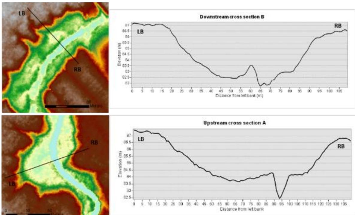
Figure 14 Cross-sections extracted from the LiDAR showing a clear ancient meander in the upstream and downstream reaches of RM.
