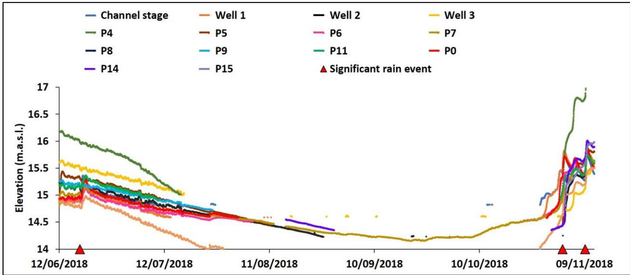
Figure 36: Channel, groundwater levels and significant rain events as a time series for the summer/fall period (including piezometers added) taken at the downstream gauging station at PPauB.
