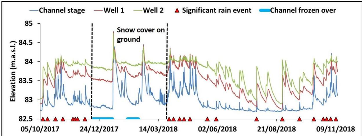
Figure 38: Channel, groundwater levels and significant rain events as a time series over the study period taken at the upstream gauging station at RM left bank.
