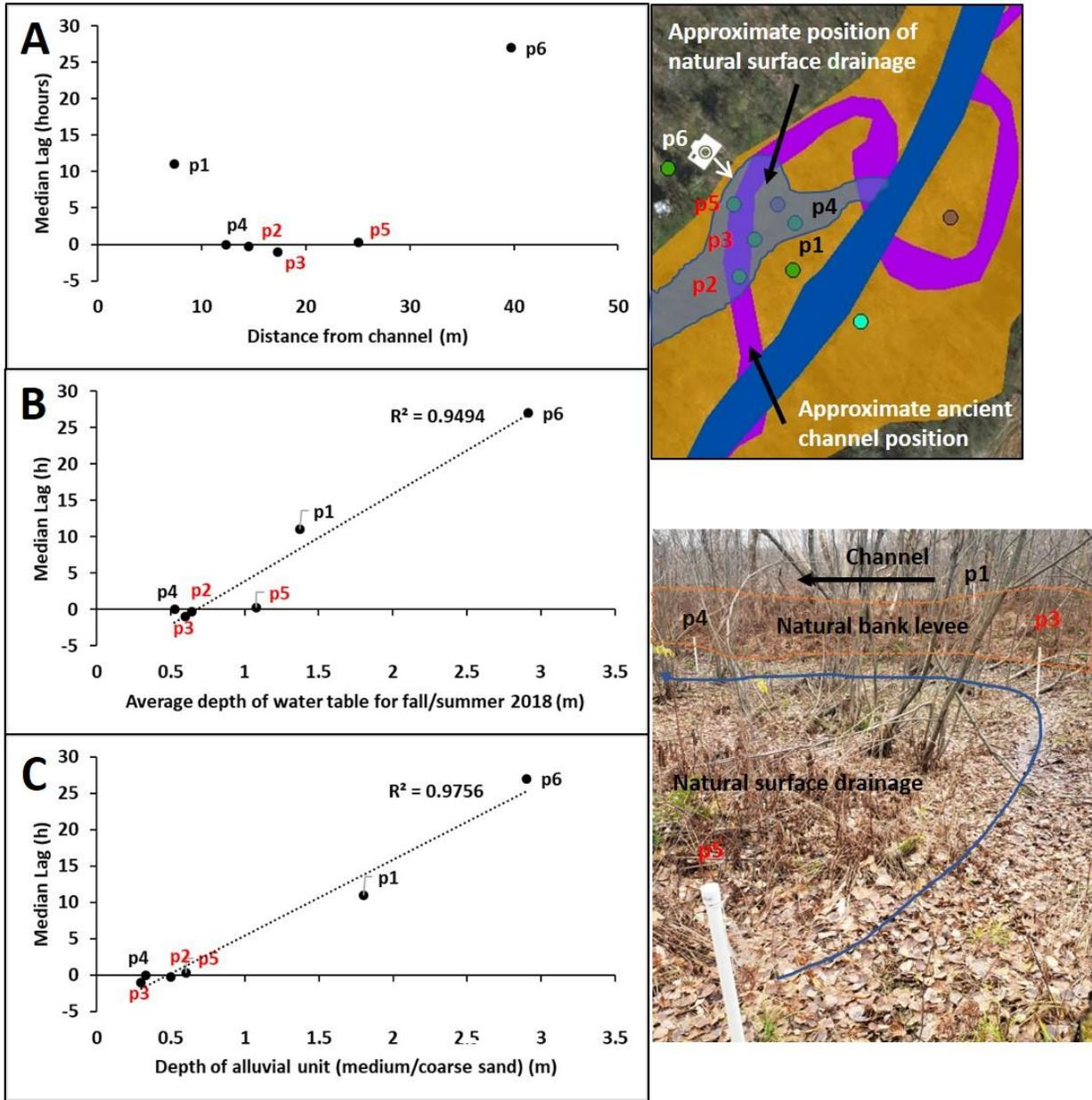
**Figure 45: Examining differences in lag times between wells/piezometers for RM MID against A) distance from channel, B) average depth of the water table, C) depth of alluvial unit. Top right shows planform view of site and piezometer positions and bottom right photo shows local topography.**
