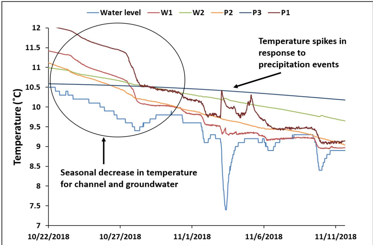
Figure 57: Zoom in of Temperature response to a series of fall floods (3 precipitation events) for RM UP.
