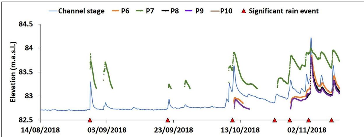
Figure 41: Channel, groundwater levels and significant rain events as a time series for the fall period (including piezometers added) taken at the upstream gauging station at RM right bank.
