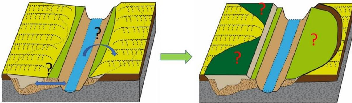
**Figure 3: Conceptual model of artificially abandoned meander due to channel straightening illustrating potential hydrological connections and restoration targets.**
