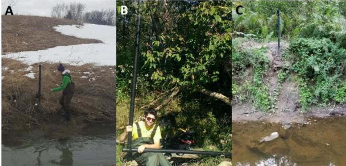
**Figure 22: ABS pipes allow for easier access to loggers during readout at DF A), example of L-piping to be installed at RM B), finished installation of L-pipe at RM C).**
