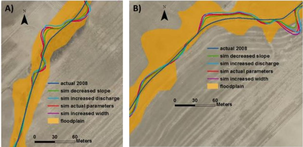
Figure 69: RVR Meander results for DF simulating actual and adjusted parameters over 50 years (2058) for A) upstream section, B) downstream section.
