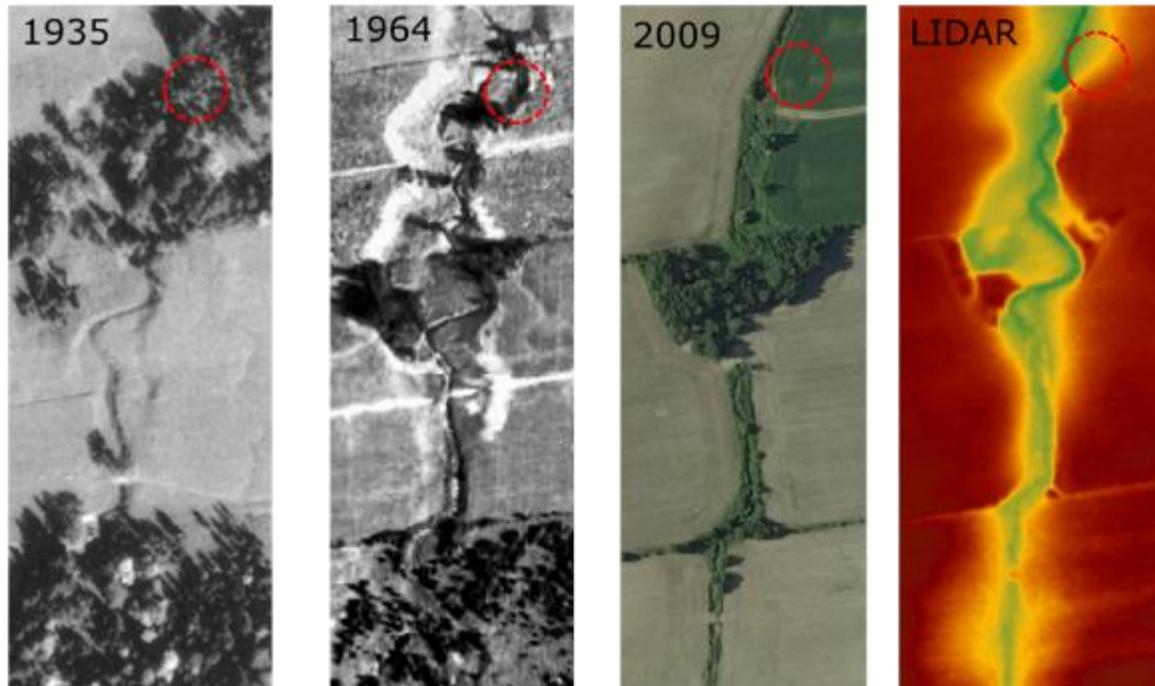
**Figure 8 : Historical air photography and LiDAR showing a clear meandering pattern in both 1935 and 1964 while the stream has a straightened pattern in 2009. Gradual deforestation is also observed from 1935 to 2009 and meander scars are visible in the LiDAR. The dashed circle shows the site where groundwater monitoring devices were installed.**
