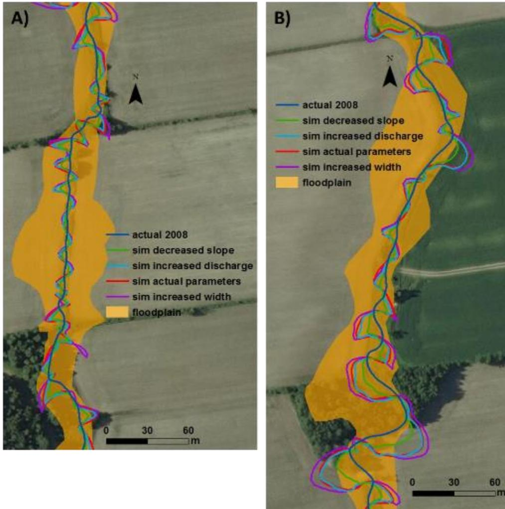
Figure 71: RVR Meander results for PPauB simulating actual and adjusted parameters over 20 years (2028) for A) upstream section, B) downstream section.
