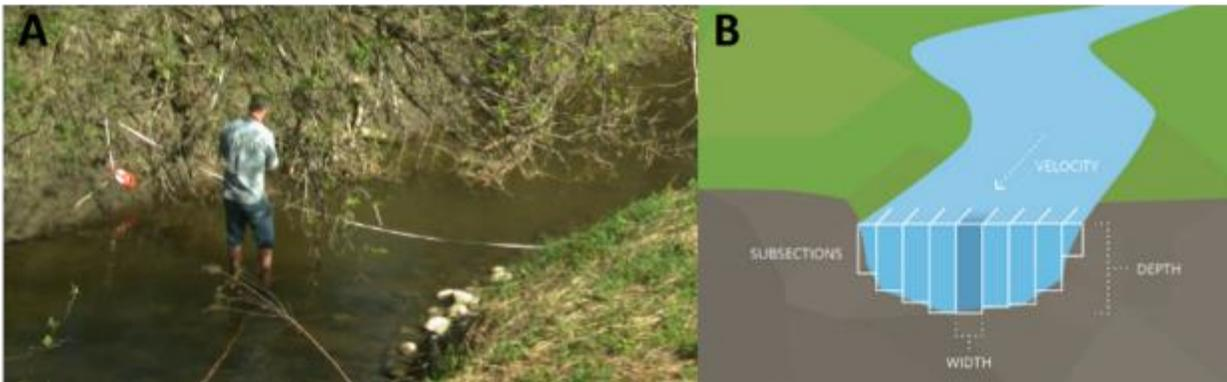
**Figure 23: Example of discharge measurement taken at RM A), and illustration of panels B) (photo credit: Fondriest Environmental, Inc.).**
