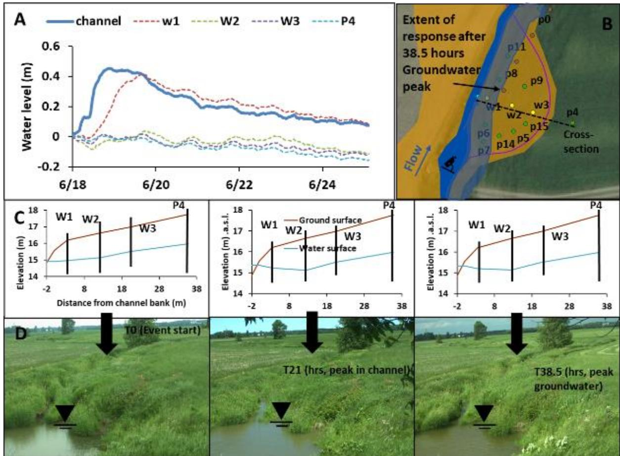
Figure 48: Hydro(geo)logic response of PPauB to a moderate summer rain event. A) water level response to the event (relative to initial elevation), B) Planform view of meander and cross-section placement, C) cross-sections of water level and ground surface at 3 times during event (start, channel peak and groundwater peak), D) photos captured from field camera for the same time steps.
