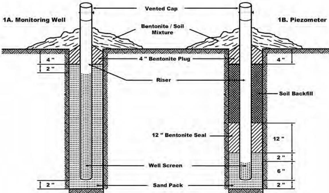
Figure 29: Schematic diagram of installed monitoring well A) and piezometer B). From Washington State Department of Transportation, [www.wsdot.wa.gov/sites/default/files/2017/07/24/Env-Wet-InstallMonWellsPiezometers.pdf](http://www.wsdot.wa.gov/sites/default/files/2017/07/24/Env-Wet-InstallMonWellsPiezometers.pdf). Note: the values of depth and width shown here are to provide an example, actual installation values are site specific depending on the depth of the basal unit (see below).
