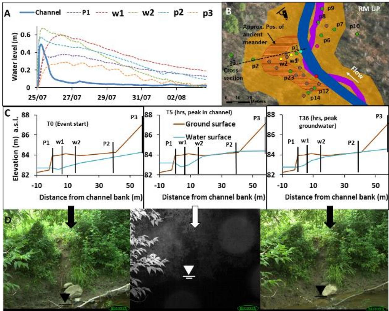
Figure 47: Hydro(geo)logic response of RM UP site to a moderate summer rain event (Table 6. event 16). A) water level response to the event (relative to initial elevation), B) Planform view of meander and cross-section placement, C) cross-sections of water level and ground surface at 3 times during an event (start, channel peak and groundwater peak), D) photos captured from field camera for the same time steps.
