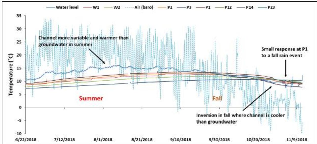
Figure 56: Summer/Fall time series of temperature for RM UP for channel and well/piezometers
