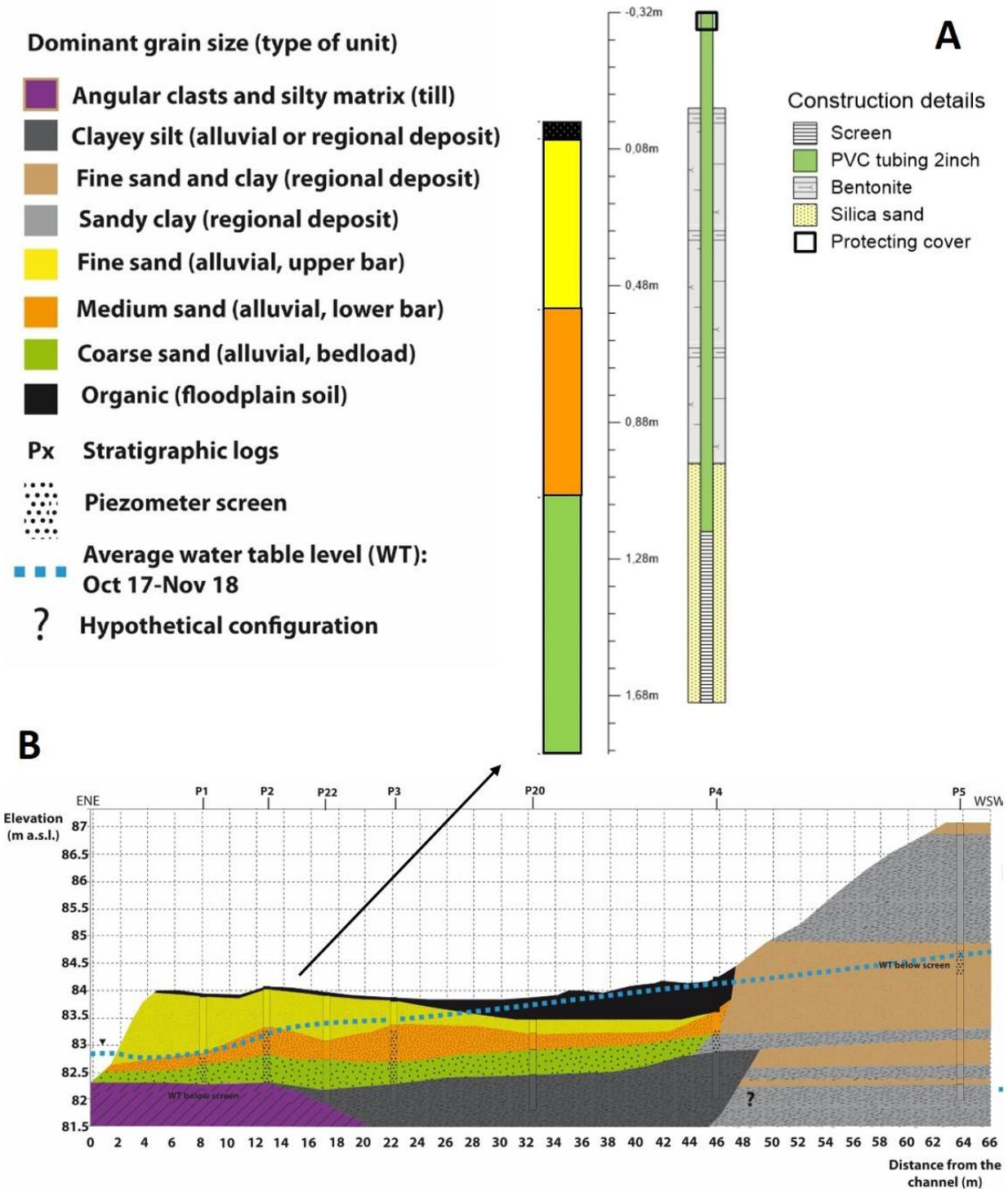
Figure 21: A) Example of borehole view layout for a stratigraphic log obtained at RM – P2; B) example of cross section view of an ancient meander at RM upstream.
