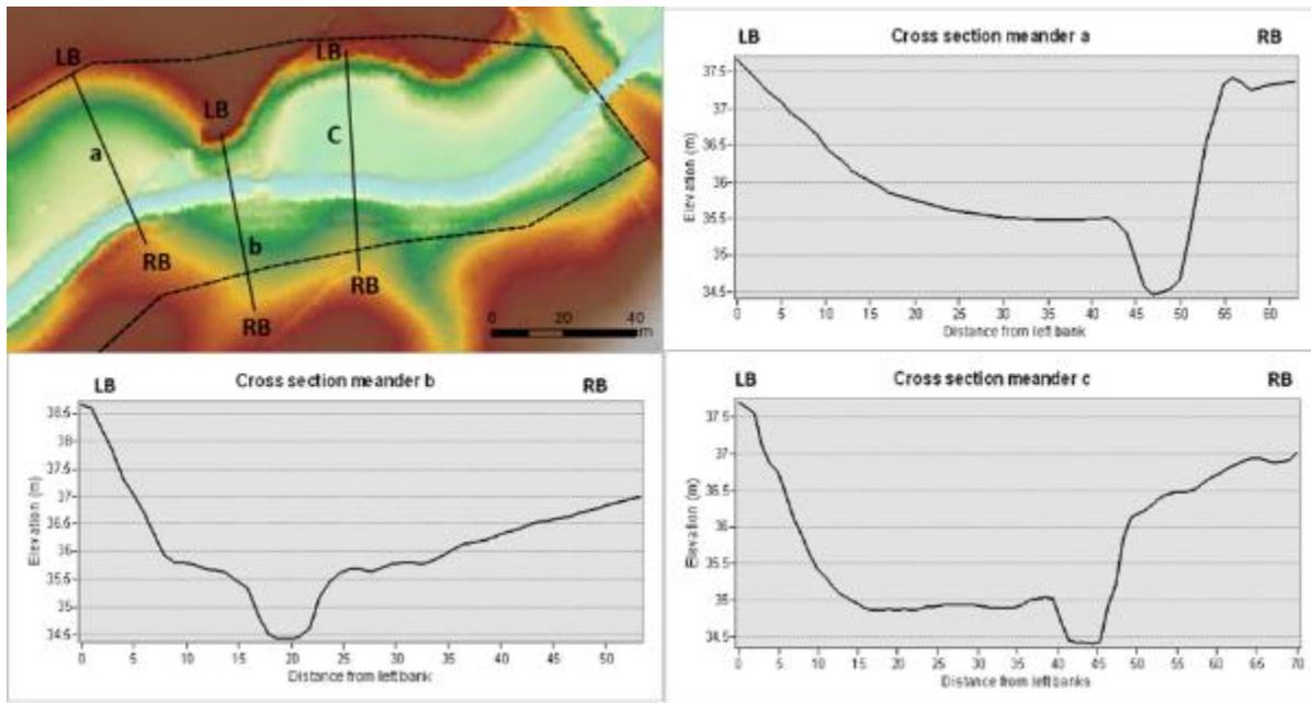
**Figure 7 : Three cross sections extracted from the LiDAR clearly showing ancient meanders in the downstream reach of Branch 53 of the Des Fèves River.**
