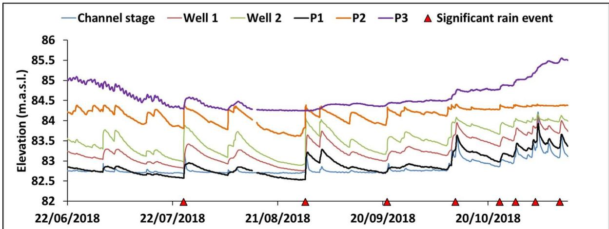
Figure 39: Channel, groundwater levels and significant rain events as a time series for the summer/fall period (including piezometers added) taken at the upstream gauging station at RM left bank.
