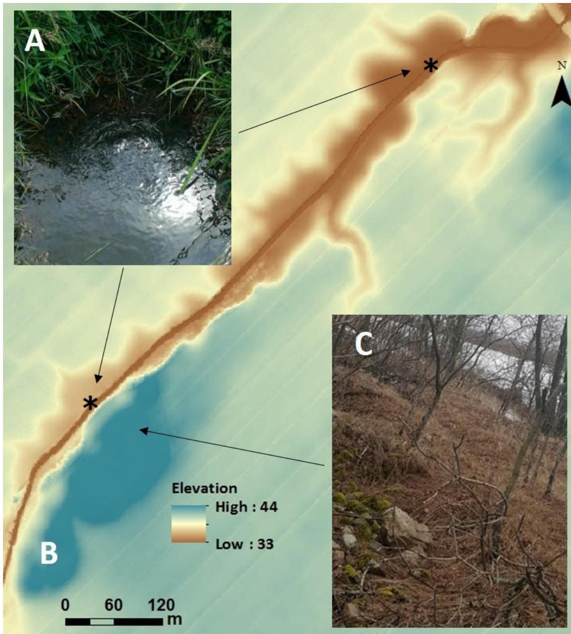
Figure 31: Example of groundwater resurgence point at DF A), drumlin clearly visible in the LiDAR B), cobble sized glacial till on floodplain C).
