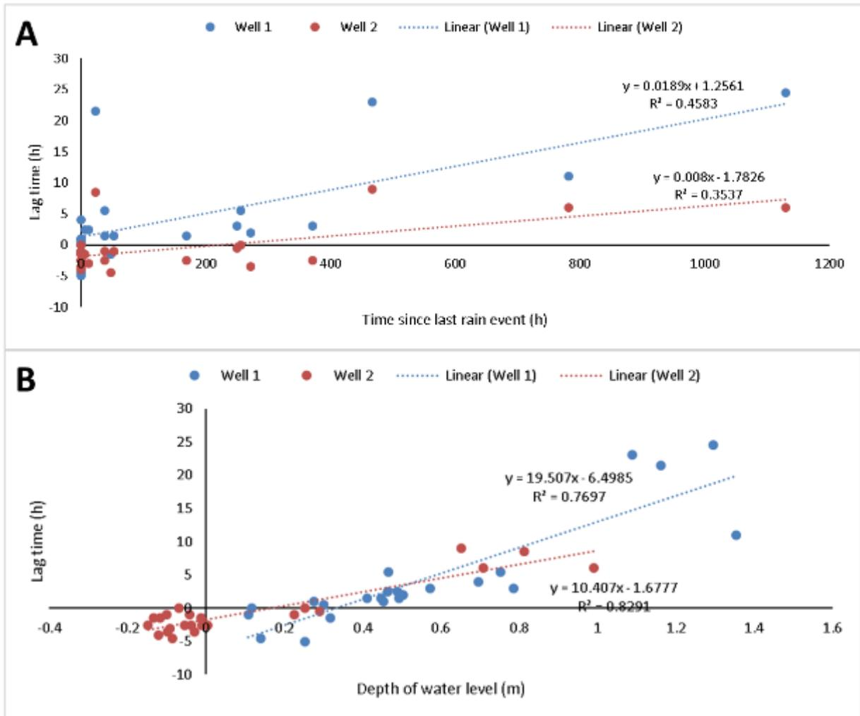
**Figure 43: Lag time response of wells installed at RM UP site to all 23 precipitation events plotted against time since last rain event A), and initial depth of water at the respective well B).**
