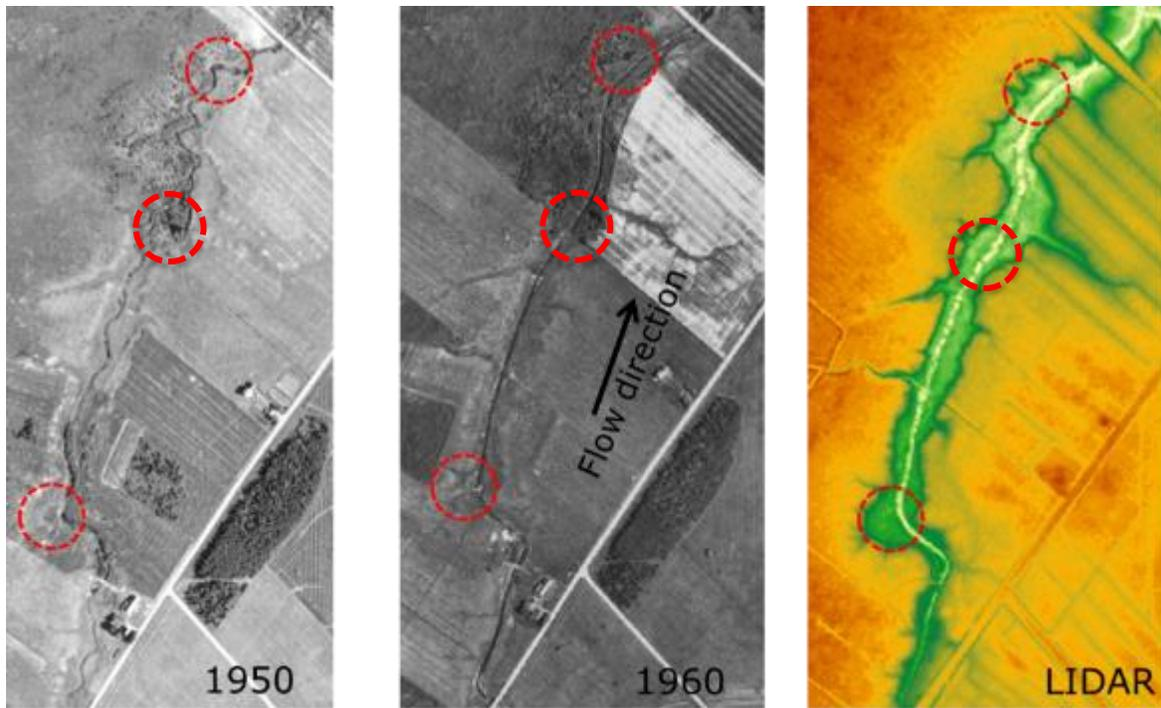
**Figure 11 : Historical air photography showing a clear meandering pattern in 1950 and a straightened pattern in 1960. Traces of abandoned meanders (red circles) are also visible in the LiDAR. Red circles also show sites where groundwater monitoring devices were installed.**
