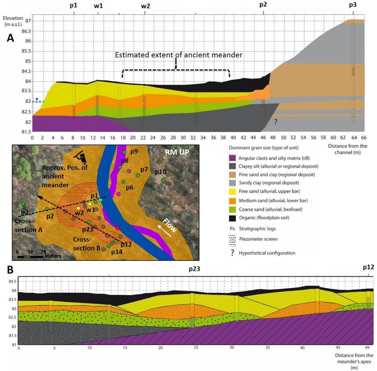
Figure 49: Stratigraphic results for RM UP. A) cross-section perpendicular to main channel, B) planform view.
