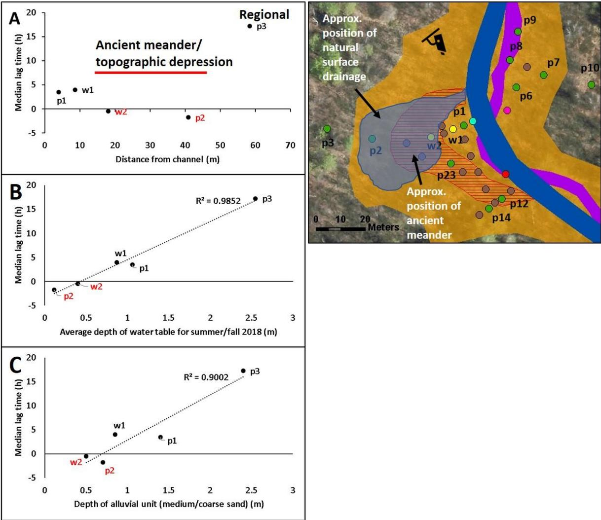
**Figure 44: Examining differences in lag times between wells/piezometers for RM UP. A) Median lag time vs. Distance from channel, B) Median lag time vs. Average depth of the water table, C) Median lag time vs. depth of alluvial unit.**
