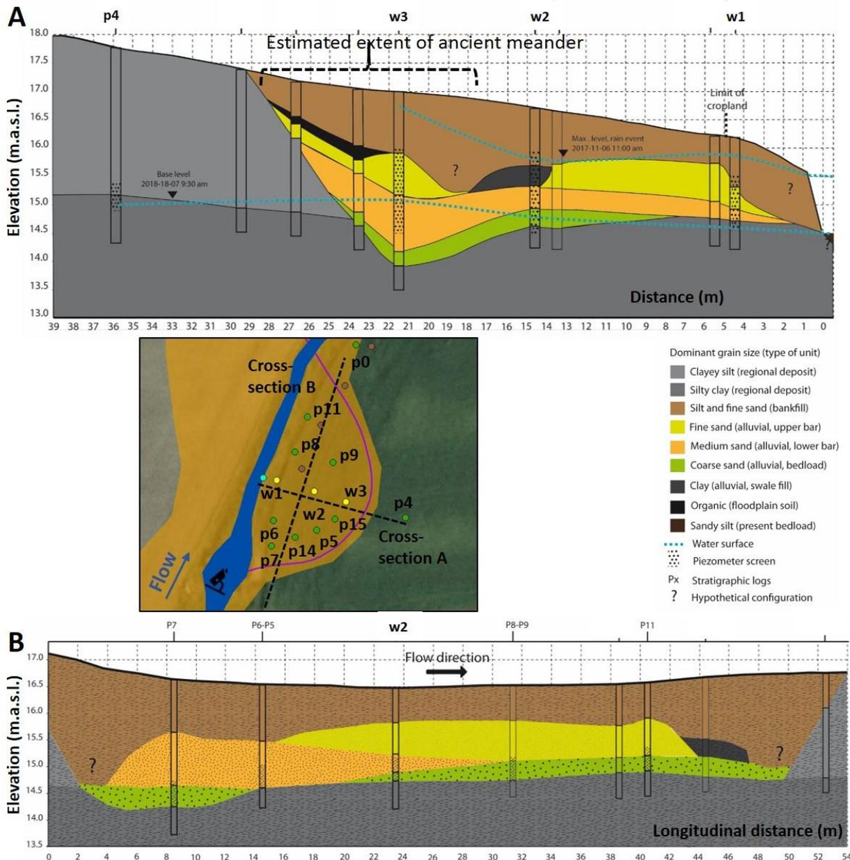
Figure 50: Stratigraphic results for PPauB. A) cross-section perpendicular to main channel, B) cross-section parallel to channel.
