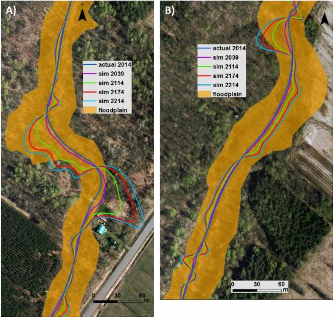
Figure 72: RVR Meander simulation results for RM using the actual input parameters for A) upstream section, B) downstream section.
