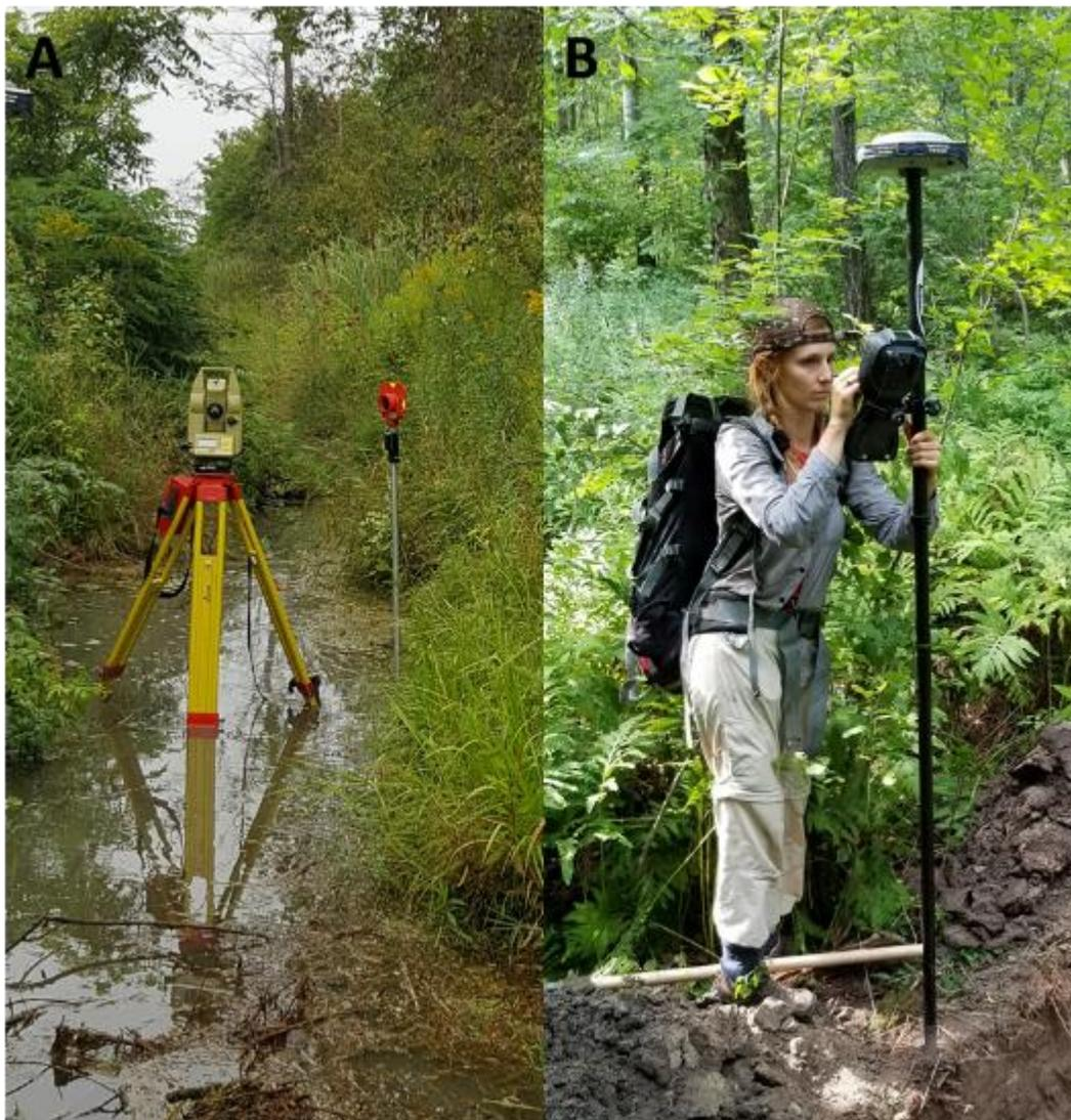
**Figure 18: Total station setup at DF A), and dGPS during a survey of RM B).**
