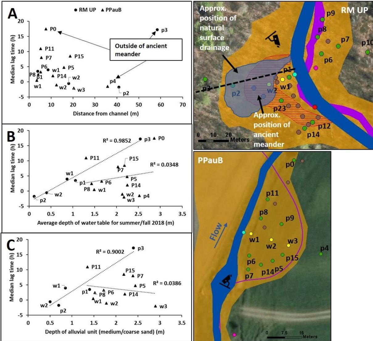
Figure 46: Results from PPauB contrasted with those for RM showing no trend between lag time and A) distance, B) average water table depth or C) depth of alluvial unit. . Note: median lag time for PPauB is based on only 1-3 values as many instruments didn't yield a significant lag time and there are few significant events.
