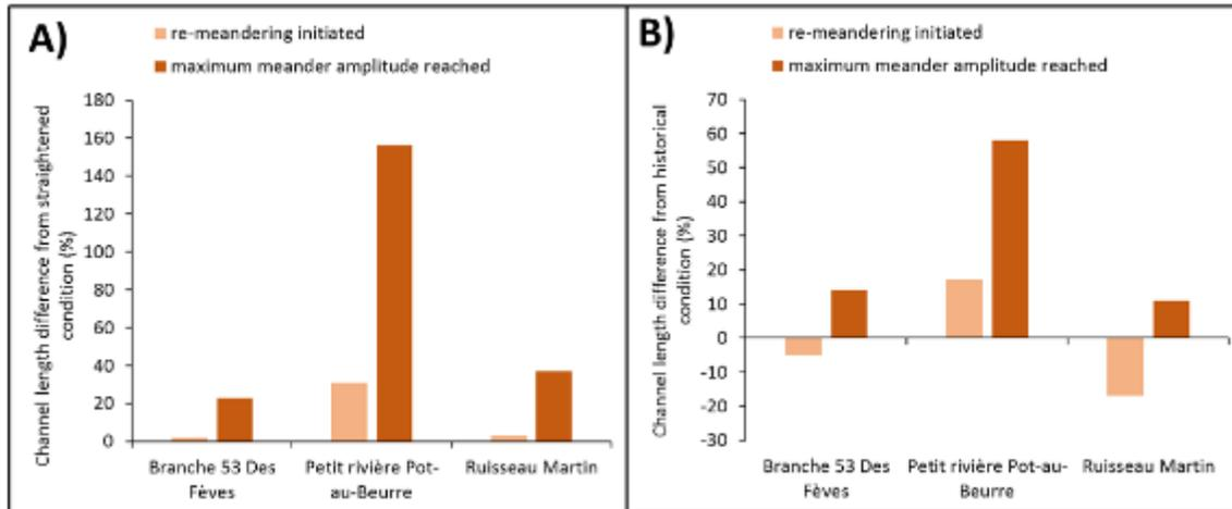
**Figure 75: Comparison between sites of the magnitude of difference for total channel length when re-meandering was initiated and maximum meander amplitude was reached. A) Percent difference between simulated results and the most recent straightened condition of the site while B) Percent difference between simulated results and the historical, pre-straightened context.**
