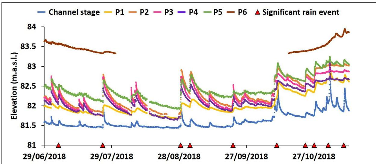
Figure 37: Channel, groundwater levels and significant rain events as a time series for the summer/fall period (including piezometers added) taken at the midstream gauging station at RM.
