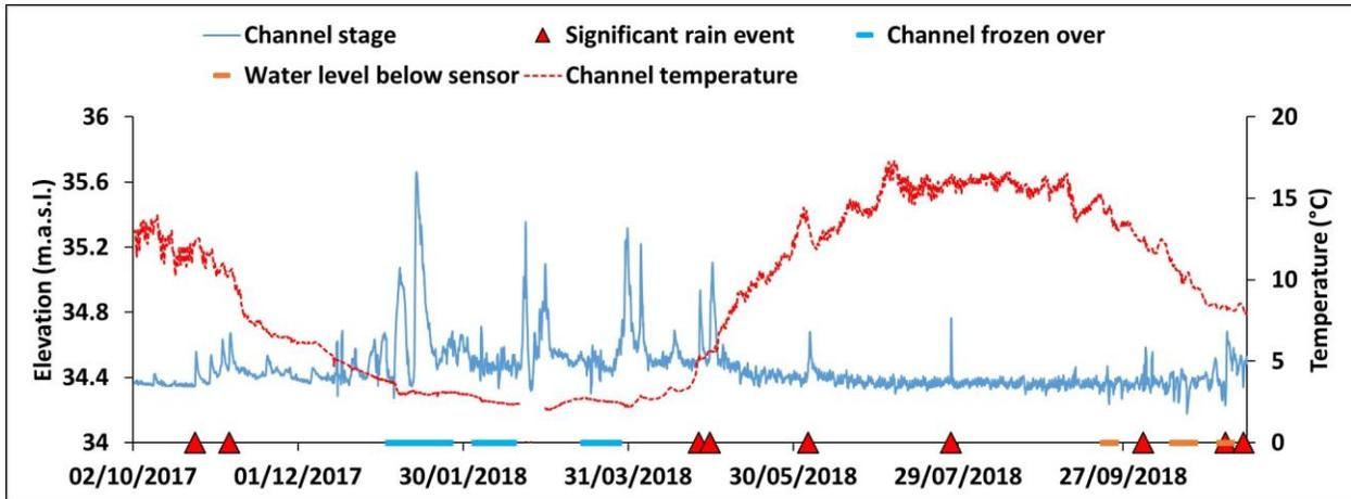
Figure 34: Channel stage (blue line) and temperature (red dashed line) as a time series over the study period taken at the downstream gauging station at DF. Significant rain events are at the start of each event.
