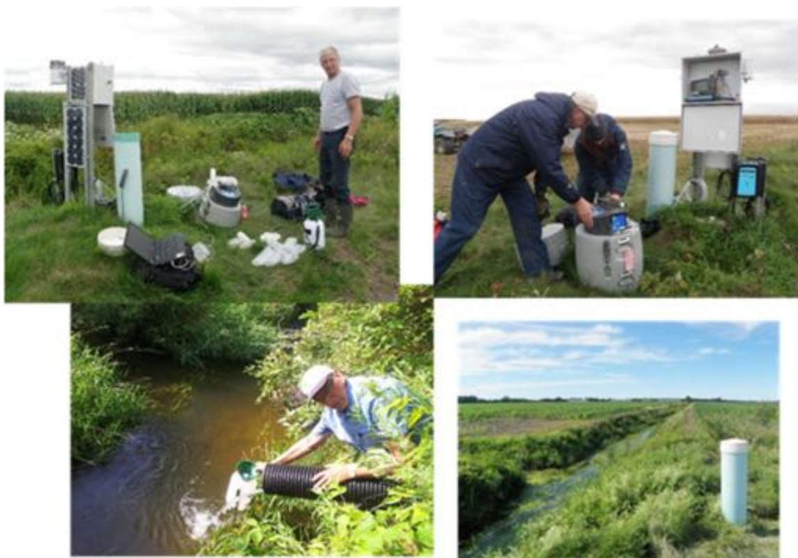
Figure 4-12. Monitoring stations of the subsurface drain collectors.
