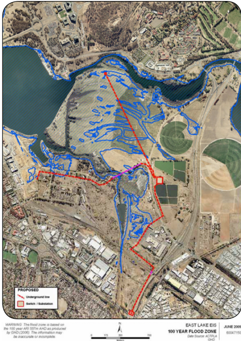
Figure CS1.3 The one in a 100 years flood zone of Jerrabomberra Creek 8
