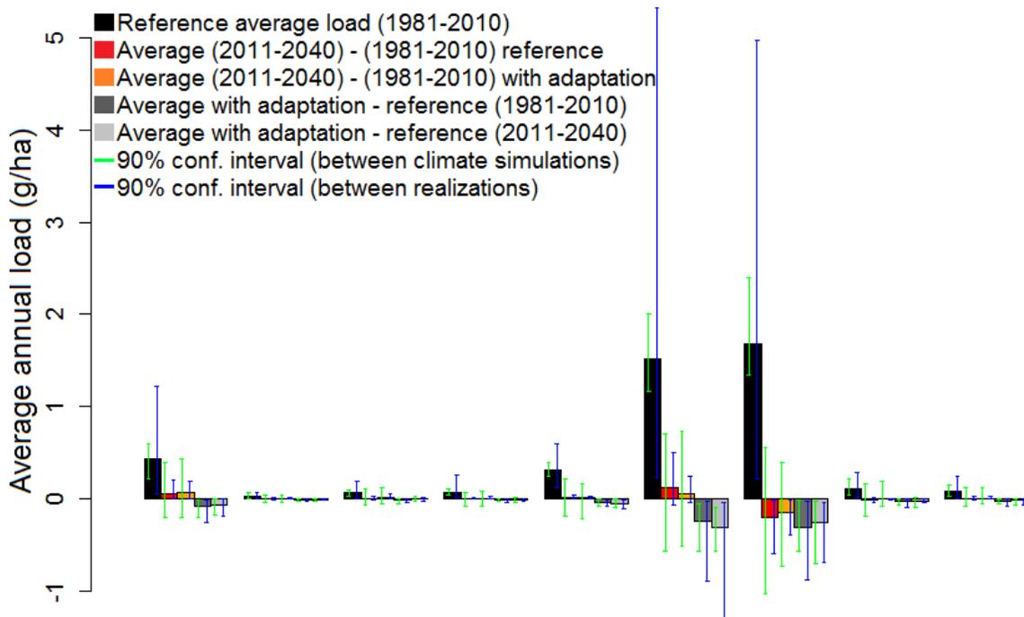
Figure 12. Impact of the adaptation measure (no application the day before rain) and climate change on the runoff load of dissolved phosmet, assessed on the 30-year averages for the nine sites simulated.
